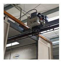
**Cab Puller** The cabin, by dragging the sling beams within the cabin, improves work efficiency, thus relieving the painter, who no longer has to move them manually.
