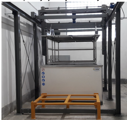
System wannowy do strippingu
