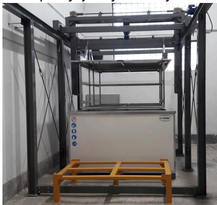
System wannowy do strippingu
