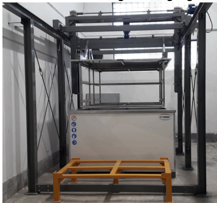
System wannowy do strippingu
