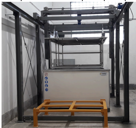
System wannowy do strippingu
